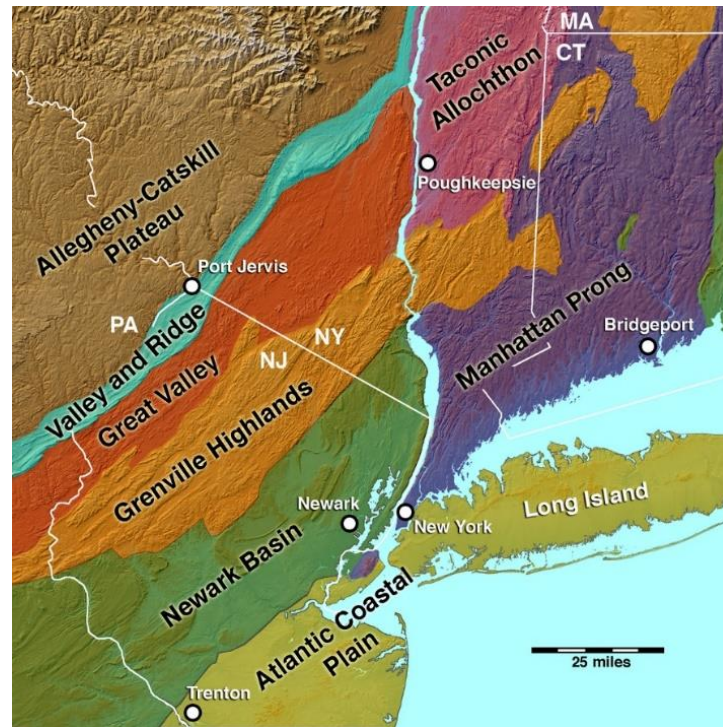
Figure 2 - Physiographic diagram showing the major geological provinces in southern New York, northern New Jersey, and adjoining states. The Manhattan Prong is shown in purple. (From Bennington and Merguerian, 2007.)
