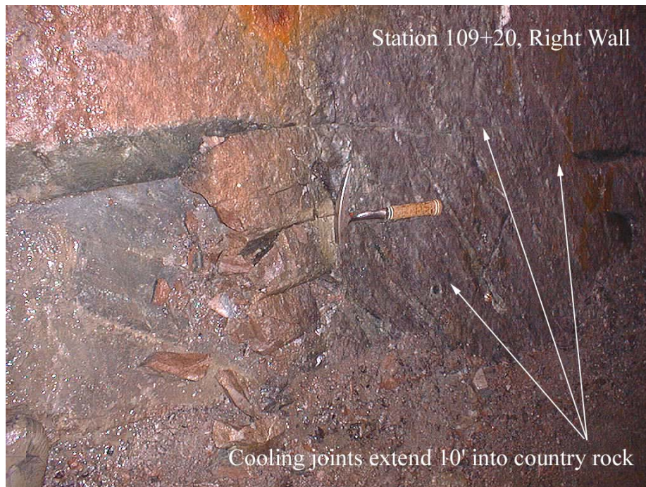
Figure 5 - Cooling joints in rhyodacite formed perpendicular to the dike margin (dike # 1) and extend over 10 feet (parallel to hammer handle) into surrounding amphibole gneiss.
