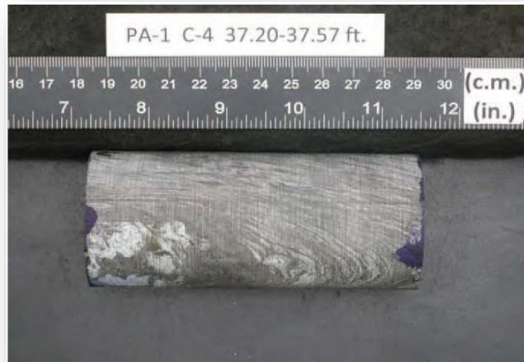
After strength testing failure.
