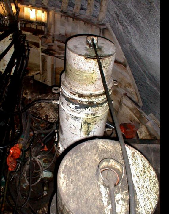
Queens Tunnel TBM 422 HP Electric Water Cooled, Three Phase Motors
