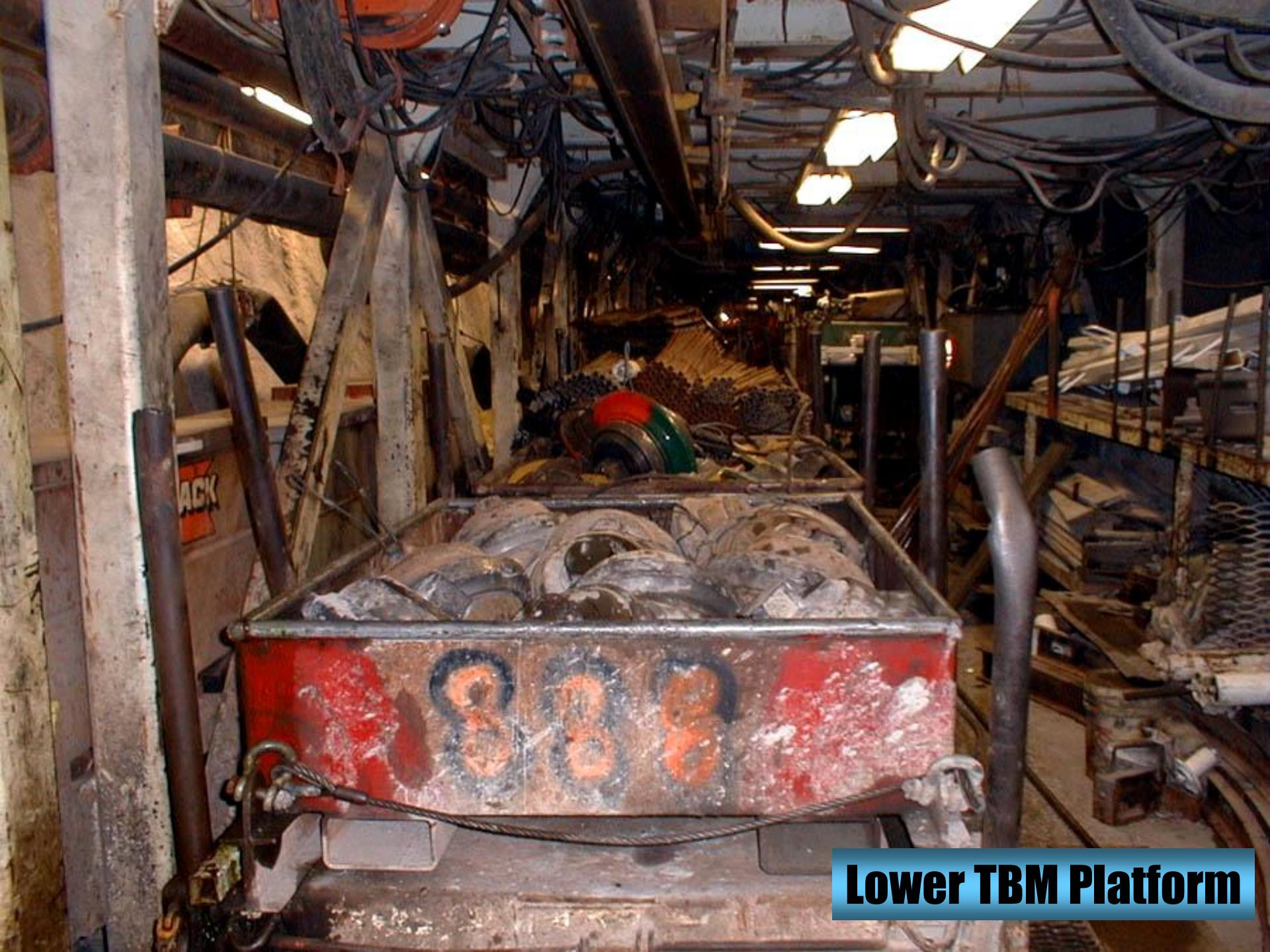
A photograph showing the interior of a tunnel boring machine (TBM) platform. In the foreground, a large metal container with the word "ROCK" painted on it is visible. The platform is cluttered with various equipment, pipes, and debris. The ceiling is supported by a network of steel beams and cables. The lighting is dim, coming from overhead fixtures.
