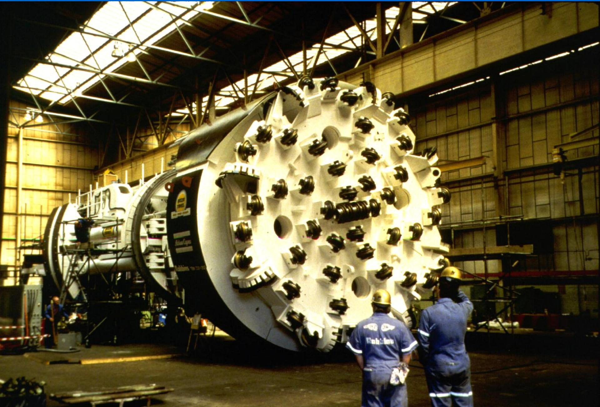
TBM excavation of ~25,000 linear feet of hard rock tunnel to 23' 2" diameter at depths of ~750'
