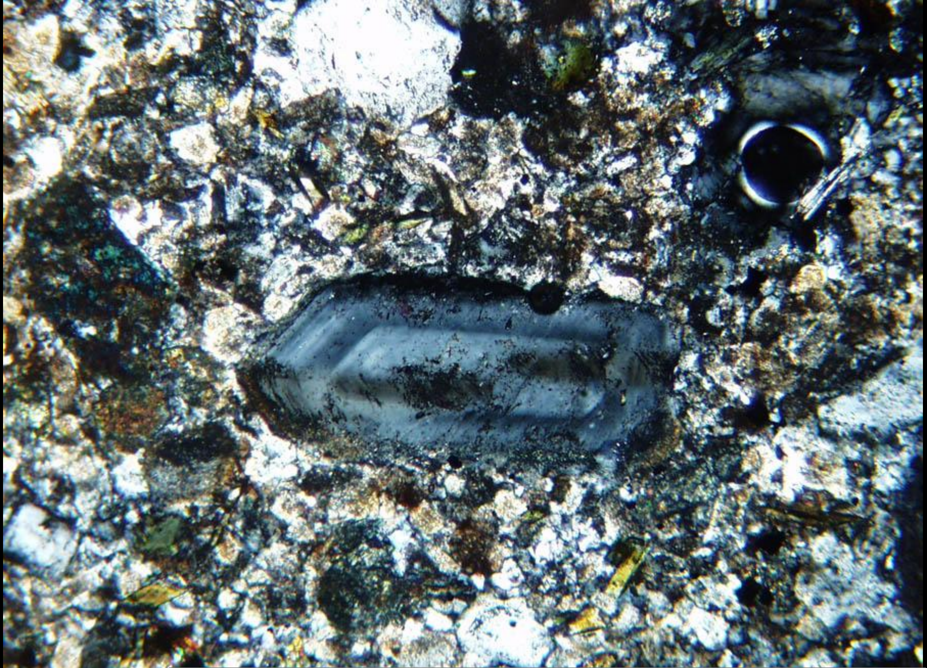
Q006C Oscillatory Zoned Plagioclase Phenocryst XN
