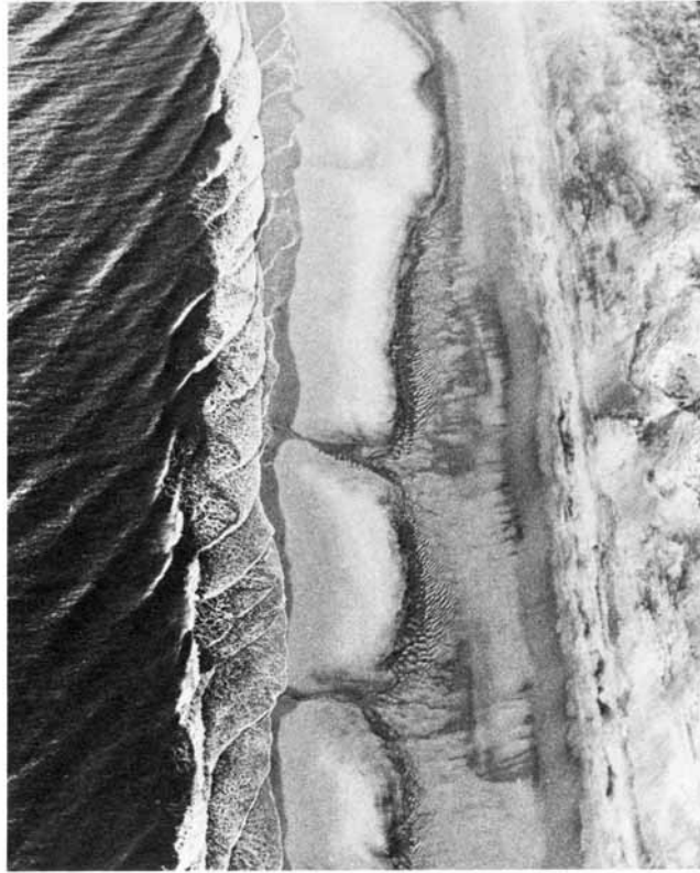
Figure 23. Intertidal circulation zone featuring ridge-and-runnel configuration viewed vertically at low tide, RMSP 09 April 1975 (Moon above Earth's equator; 2 days after apogee; 2 days before Full Moon). Two gaps cut the ridge. Transverse bedforms in runnel (long axes perpendicular to shore) indicate that the water flowed seaward. Small waves approaching obliquely from the SW (upper L) break before they are refracted. Other, less-obvious sets of waves are in sets traveling from W to E, nearly perpendicular to shore, and larger swells, approaching from the S, nearly parallel to shore. Photo by B. Caplan; From Freidman and Sanders, 1978, Fig. A-31, p. 490.)
