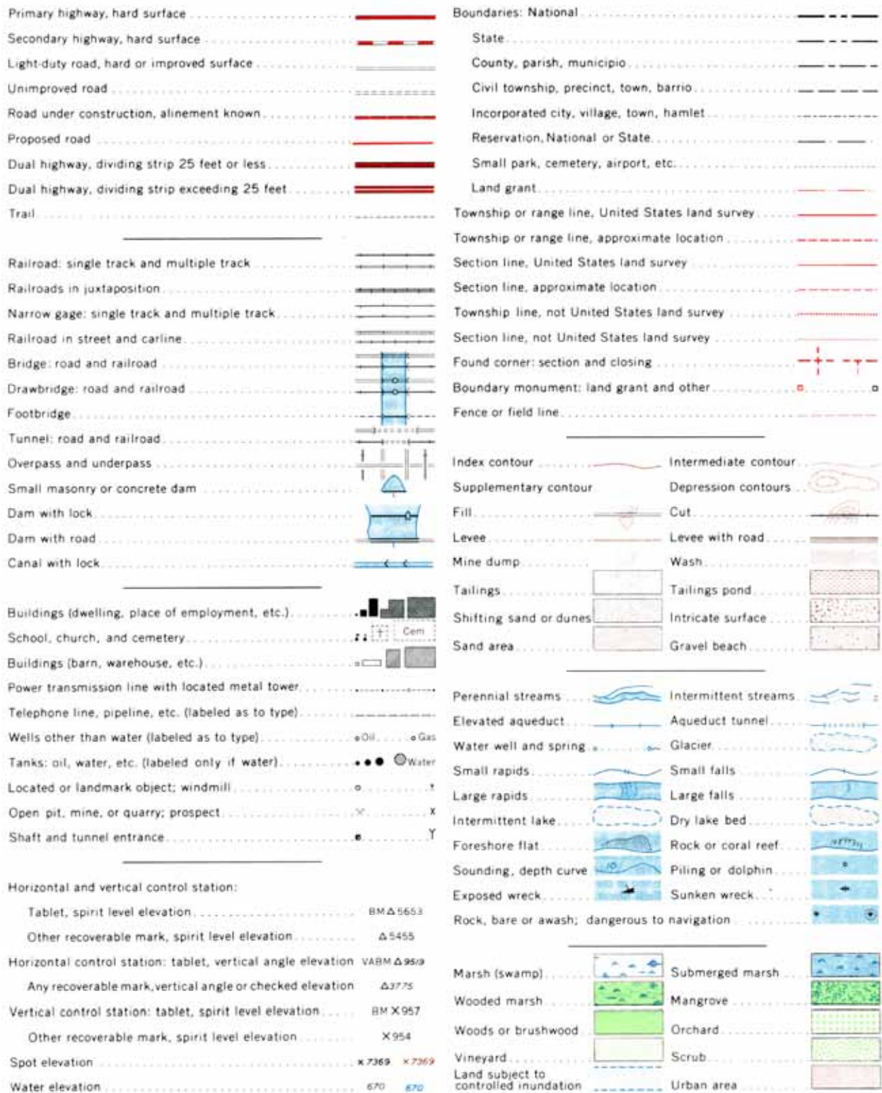
Figure 10.8 - Topographic map symbols. (United States Geological Survey.)
