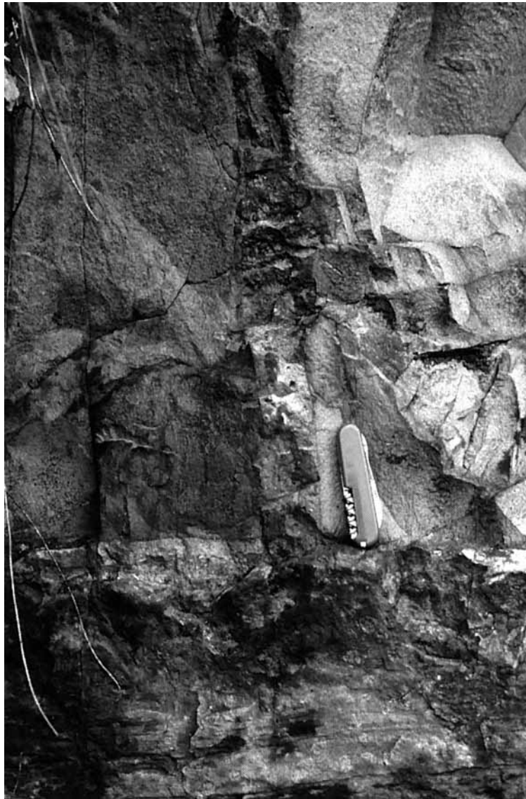
Figure 41. View of a 3-cm-thick feldspathic "clastic dike" that has intruded the Palisades chilled margin. Knife (scale) is 9 cm in length. (CM photograph.)
