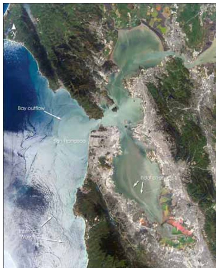
Figure 39 – Satellite image of the San Francisco Bay area showing refraction and internal waves produced by strong currents that buffet the west coast of North America in the vicinity of San Francisco. The San Andreas fault is the linear feature that trends NNW along the western California coast. Note the sediment plumes related to the Sacramento and San Joachin rivers. Clearly the satellite image indicates that the San Francisco Bay area is a drowned river mouth.
