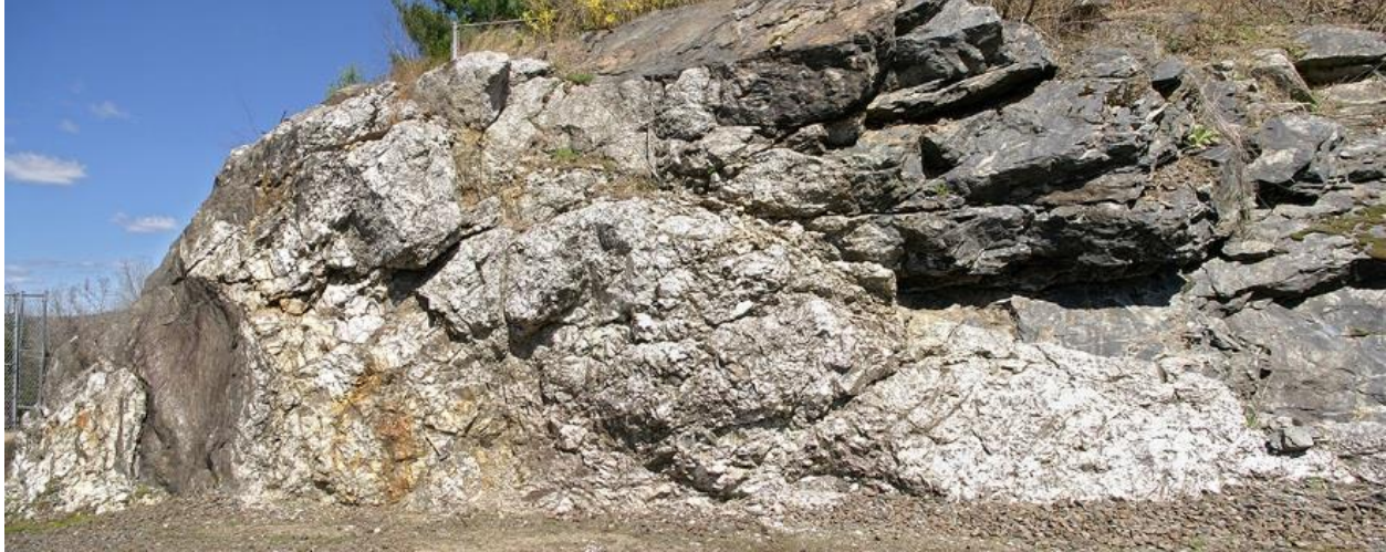
Figure 26. Pegmatite on access road adjacent to spillway cut. It intrudes gray The Straits Schist. (H. Moritz photo.)
