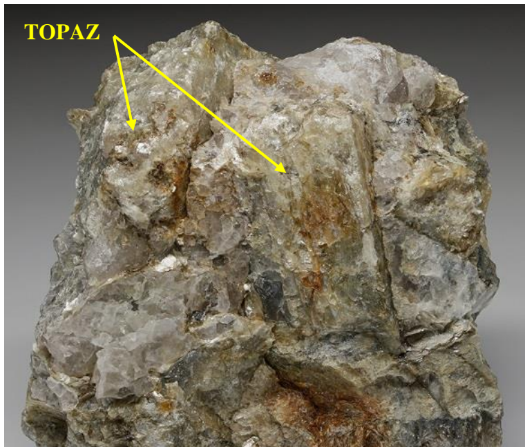
Figure 9. Subhedral topaz crystals (pale yellow-green with micaceous coating) in quartz (colorless glassy) from the core zone of a typical vein. (H. Moritz photo.)
