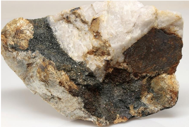
Figure 38. Sample of the contact between discordant, white, bull quartz (top center) and schist (lower left). Dark green, fine-grained chlorite (commonly with fluorapatite and magnetite) lies in between them, with a flat, undeformed, euhedral ilmenite crystal at right, rooted in the contact. The very brittle ilmenite crystals are mostly found as fragments in mine waste. (H. Moritz photo.)
