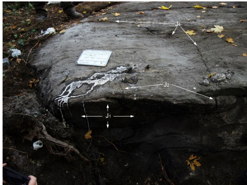
Figure 21 – Post pulse #2 view of bedrock showing internal fracturing and failure along the J_1 , J_2 and J_4 joints. Rocks were readily peeled from exposure by mechanical means and methods. (Dukelabs image taken 17Nov21.)
