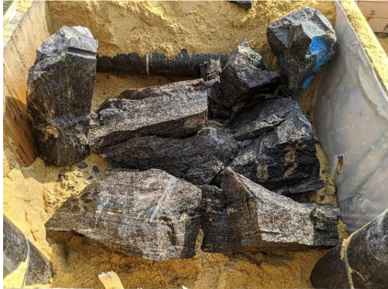
Figure 13B - Sample G3 after pulling apart by hand (no tools).
