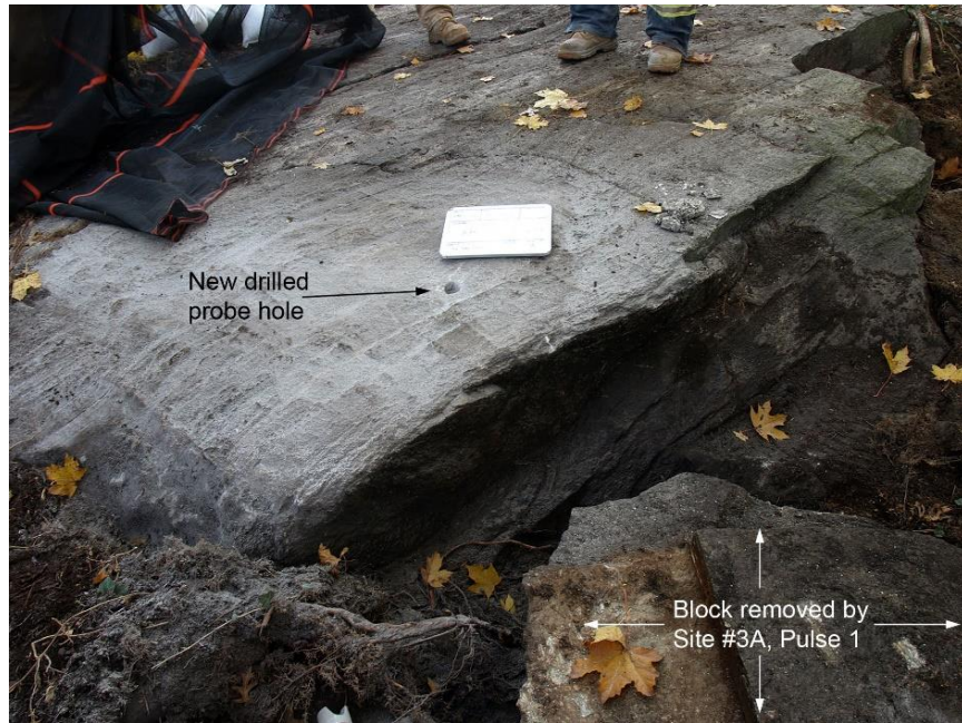
Figure 20 – View of drilled hole before placing PT probe into rock mass for second test pulse. Hole is 12” inches from newly exposed active open face which was revealed after rotating the large block from pulse #1 away from the outcrop. The newly open face is controlled by the S_1 and J_1 weakness surfaces. The effectiveness of the initial pulse can be seen by comparing this view with previous images of the #3A site (Figure 18). (Dukelabs image taken 17Nov21.)
