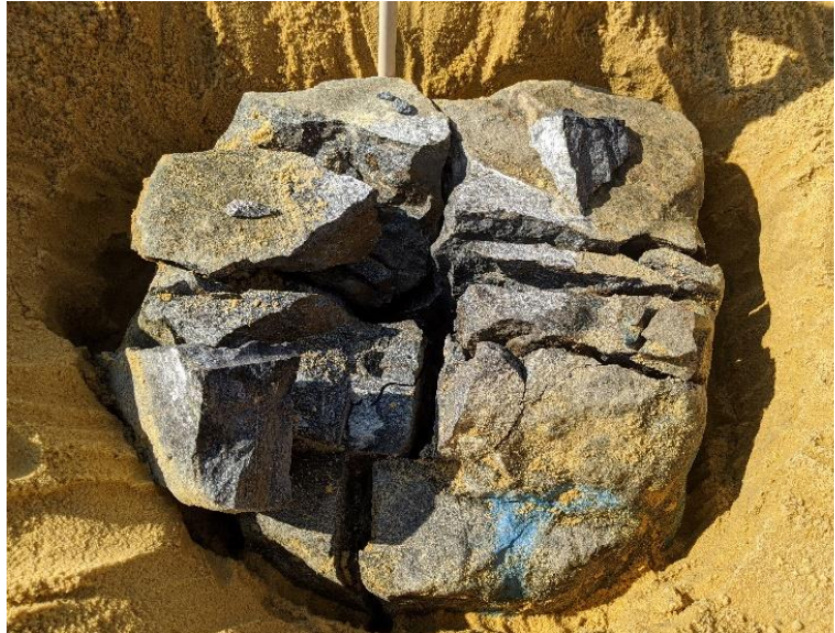
Figure 11B - Sample G4 after pulse and unburying.
