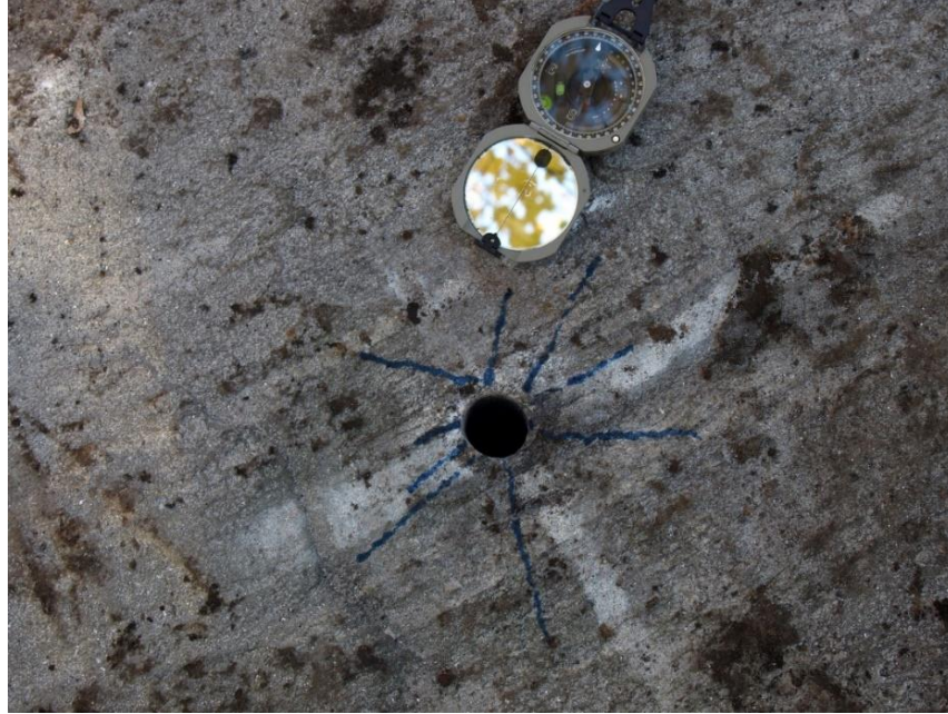
Figure 25 – View of radial fractures subtended around pulsed drill hole after pulse #3 at site #3B. Note how the incipient fractures (drawn blue lines) preferentially parallel the S_1 foliation and parallel J_1 joints, both trending about N35^\circ E . Center line of compass points (upward) toward true North. Overnight relaxation of rock mass had taken place. (Dukelabs image taken 18Nov21.).
