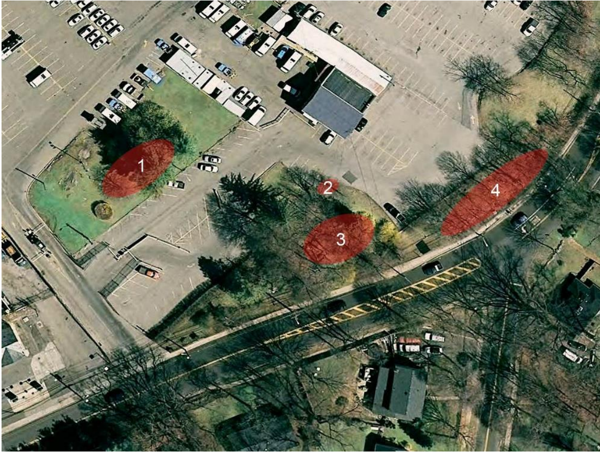
Figure 16 – View of four main outcrop areas consisting of NE-trending migmatitic gneiss, granofels, schist and minor amphibolite of the Hartland Formation, a common constituent of NYC bedrock. Site #3 was selected for reasons of equipment accessibility and support and ability to plan for three modes of plasma tool field use to best simulate actual trench construction in solid, confined rock ledge. Site #3 is also desirable for the lack of post-excavation visual disturbance as the area is tree-bound and well-vegetated. (Google Earth Pro image, 2021.)
