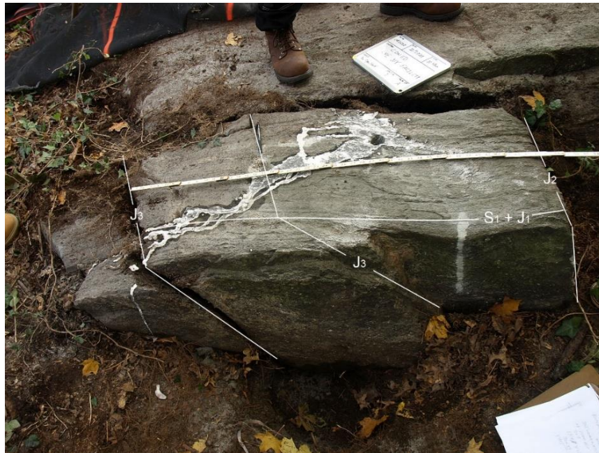
Figure 19B – Same view as above Figure 19A showing the outline of preferential breakage planes S_1 , J_1 , J_2 and J_3 that surround and cut through the large block that was displaced by pulse #1. The block was bounded along the bottom and top by sub-horizontal J_4 sheeting joints. (Dukelabs image taken 17Nov21.)
