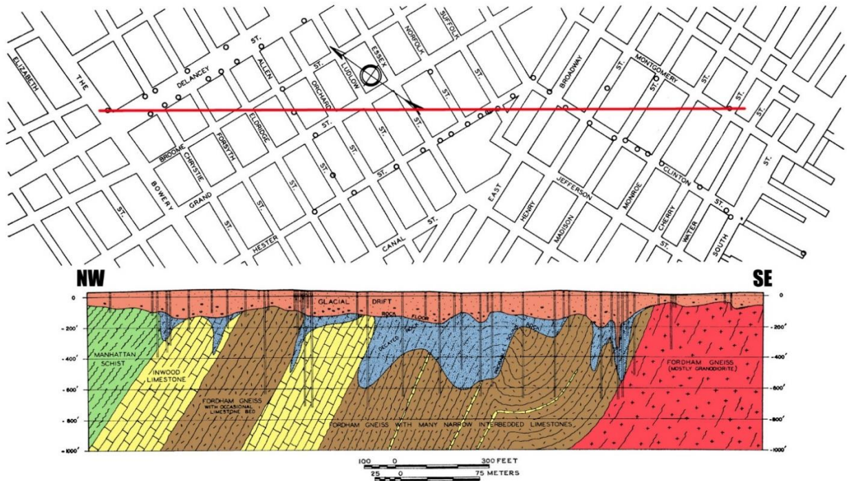
Figure 5 – NW-SE profile section in southeastern Manhattan Island showing steeply inclined Proterozoic and Paleozoic bedrock units and an overlying blanket of Pleistocene glacial drift that averages over 100' in thickness. Note also the deeply weathered bedrock (blue) at the top of rock. Line of section in red. (Adapted and colored from Berkey, 1933a, b).
