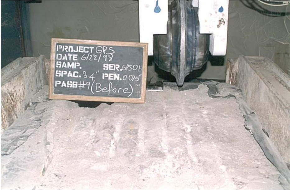
Figure 10 – View of a 19-inch cutter on LCM.
