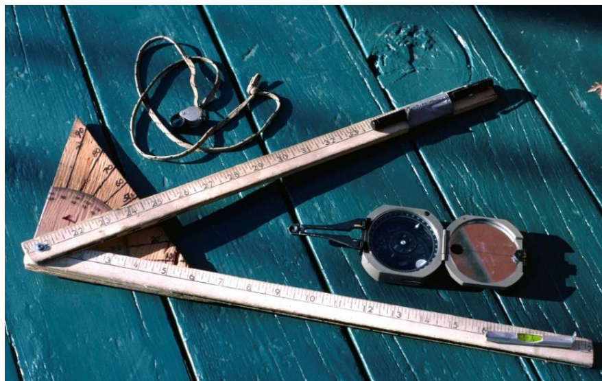
Figure 2 – Mechanism used for measuring strike of features exposed on both tunnel walls at springline and comparing to surveyed invert orientation. Dips were measured using Brunton compass and verified by cartographical calculations from map geometries.
