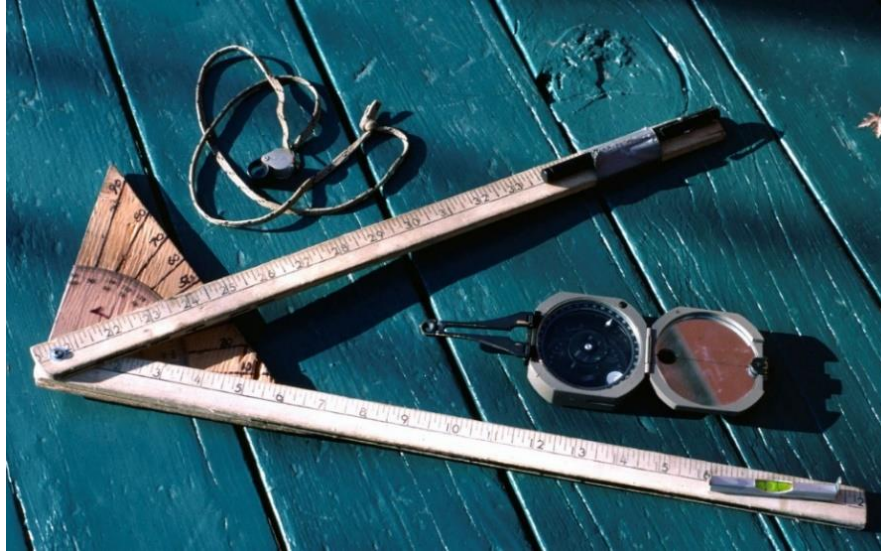
Figure 18 – In-house mechanism used for measuring strike of features exposed on both tunnel walls at springline and comparing to surveyed invert orientation. Dips were measured using Brunton compass and verified by standard cartographical calculations from map geometries.
