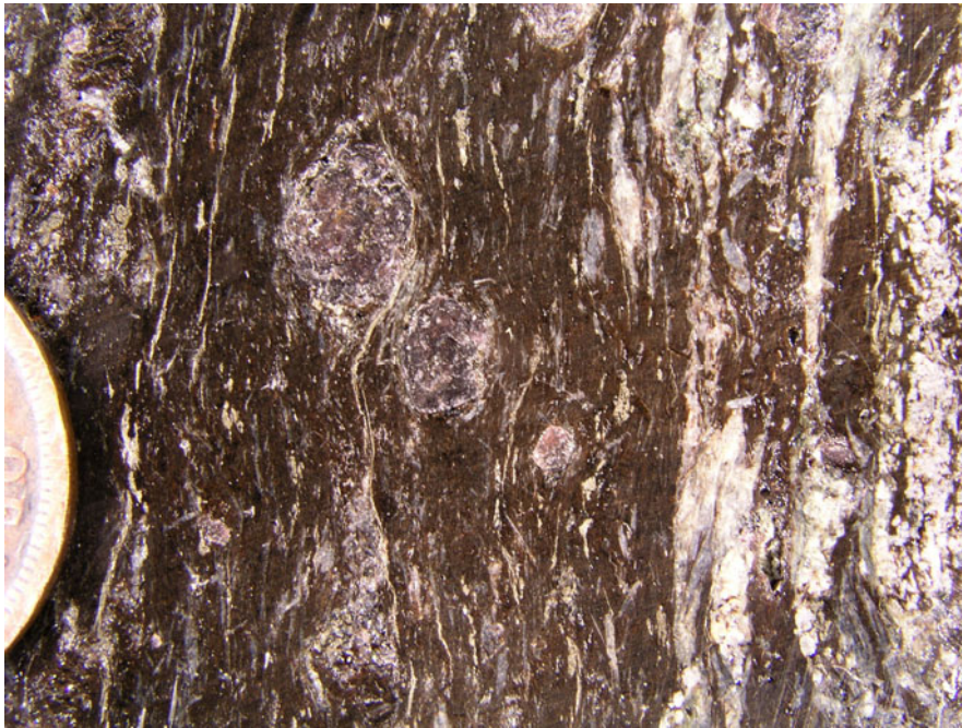
Figures 5A, 5B – Broken surface of rock core from Boring B-5 showing typical Manhattan Schist (Unit \epsilon -Om) found along the eastern edge of the site, here a massive coarse-textured muscovite – biotite - garnet schist showing a migmatic texture. Same sample (N732) as shown above in Figure 4B. In Figure 5B, close view of sawn drill core consisting of predominately Walloomsac with some intermixed Manhattan Schist from sample N734 near south center of site (Boring B-13). Note the overall flaser texture and dense, laminated fabric in the Walloomsac consisting of fine-textured red-brown biotite. Garnet and kyanite porphyroblasts are rotated and sheared and quartzofeldspathic segregations and pyrite show extreme stretching and disarticulation. This unique boring captures the mylonitic contact (St. Nicholas thrust) between the Walloomsac and light-colored Manhattan lithotypes to the left and right of the image. Edge of Indian Head cent for scale in both images.
