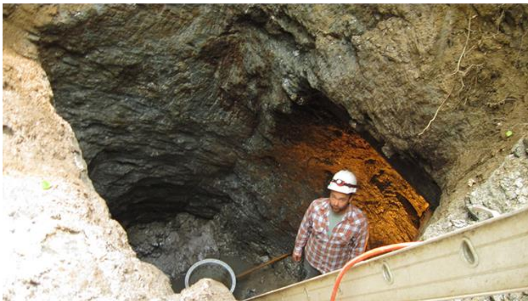
Figure 29 – Shaft #1 (sub-stop 5) after excavation. Original mine timbering is visible at the top of the short tunnel lit up behind the site owner. The schist contains emerald-green muscovite variety fuchsite, likely mistaken for malachite. (From Moritz and Merguerian 2015, fig. 43, p. C1-C27.)
