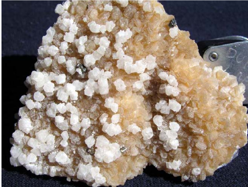
Figure 11. Photographs of some secondary minerals that infill some fracture interstices in the Queens water tunnel.
