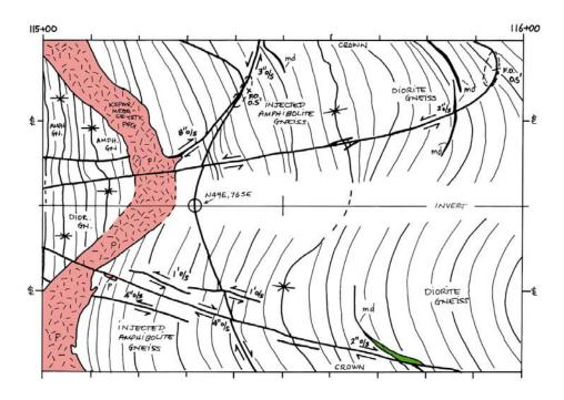
**Figure 8** – Map showing a NNW-trending left-lateral strike-slip fault of Group E that eventually cuts the tunnel invert at Station 114+90. The fault is oriented N48°W, 64° SW and is a relatively thin (~3 cm) feature. (Tunnel bearing is N41°W; Original map scale 1"=10"; tunnel diameter 23′ 2".)
