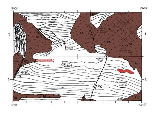
**Figure 6** – Map of migmatitic biotite garnet amphibole gneiss cut by two rhyodacite dikes. The dikes are cut by NNE-trending faults of Group D. (Tunnel bearing is N71°W; Original map scale 1"=10"; tunnel diameter 23' 2".)
