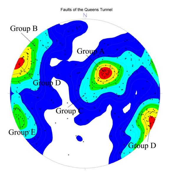
**Figure 2** – Schmidt equal-area stereogram showing the poles to 306 faults mapped in the as-built Queens Tunnel. **Group A** faults strike NW and dip gently SW, **Group B** faults are moderate to steep and strike ENE, **Group C** are subhorizontal fractures and faults, **Group D** constitutes the NNE-trending fault system of the Queens Tunnel, and **Group E** are the youngest NNW-trending strike-slip faults.
