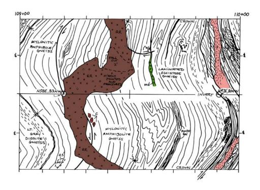
**Figure 5** – Geologic map showing truncation of N53°E, 83°NW Group B fault by a NW-trending rhyodacite dike of 4 m thickness. (Tunnel bearing is N09°W; Original map scale 1"=10"; tunnel diameter 23' 2".)
