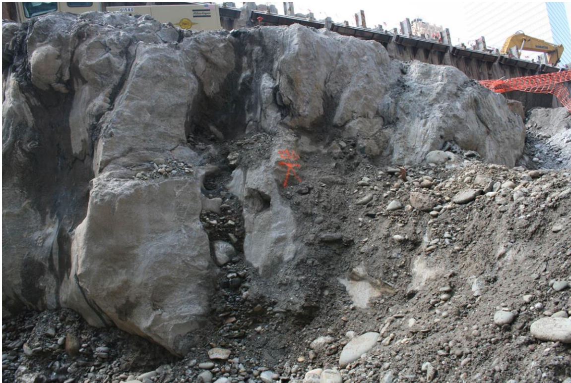
Figure 11 – Pothole filled with dense till. Spiral grooving can be seen in the bedrock. (Digital image by C. J. Moss.)
