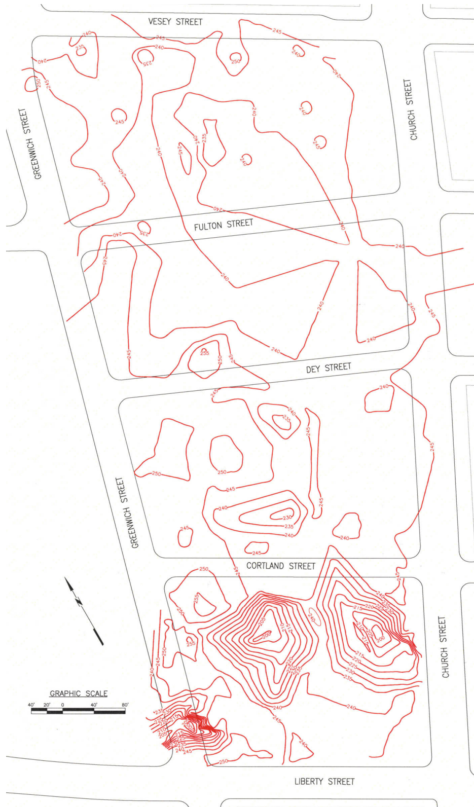
Figure 4 – Bedrock contours in the East Bathtub based on the newest borings and construction data. The valley consists of two bowl-like depressions that trend WNW before heading SW into a narrow valley that runs offsite, below Liberty Street. Elevation 300' = El +2.653' (1929 NGVD).
