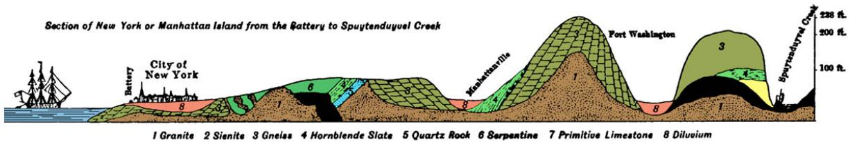
**Figure 4** – S to N profile of Manhattan, from Battery (L) to Spuyten Duyvel Creek (R), showing shape of land surface (shaded, below) and inferred geological relationships as determined by Issachar Cozzens. (Adapted from G. P. Merrill, 1924, fig. 43, p. 238; after Cozzens, 1843).
