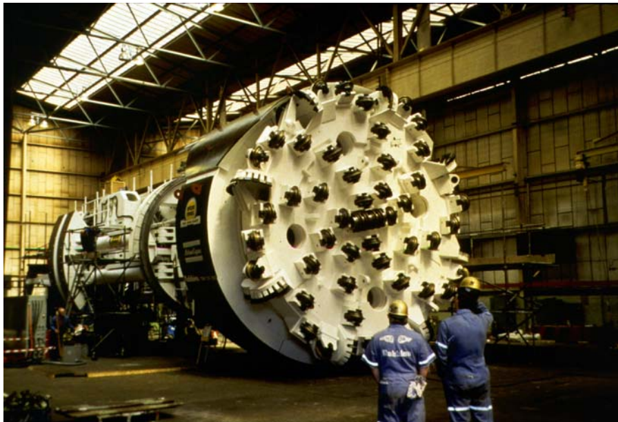
Figure 1 - The front cutterhead and thrust assembly (business-end = 84' length and 23' diameter) of the Tunnel Boring Machine that formerly operated beneath western Queens. With a total length of nearly 300', the complete machine excavates, processes, and removes the rock chipped by the cutters. The cutterhead rotates against the raw rock face with thrust applied hydraulically by mechanical contact from behind against the sides of the bored tunnel. The TBM holed through beneath Long Island City in October 1999 after three years of nearly continuous subsurface mining.
