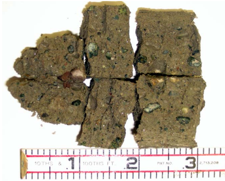
Figure 7. Sample of typical NYC area basal till taken in a split spoon sampler from lower Manhattan near the World Trade Center site. The distinctive structure and texture of the soil are typical of basal till found from many sites across the NYC area. Thin layers of till encountered in or near the base of the varved strata from the study site have the same soil structure as this sample.
