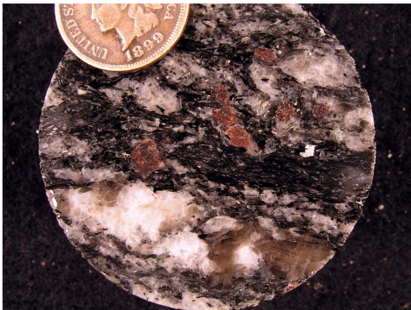
Figure 1 – Macrophotograph of sawn core of sample N751 showing vertical gneissic fabric consisting of recrystallized light-colored quartzofeldspathic layers separating contorted mica-rich layers that are injected by quartzofeldspathic segregations. Garnet porphyroblasts up to 4 mm in size overgrow the predominant metamorphic layering, indicating a younger phase of metamorphic overprinting and recrystallization.
